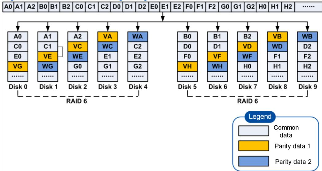
One RAID 60 array consists of multiple RAID 6 volumes. At least eight hard disks are required for RAID 60. Data is distributed on each RAID 6 volume in RAID 0 mode.
