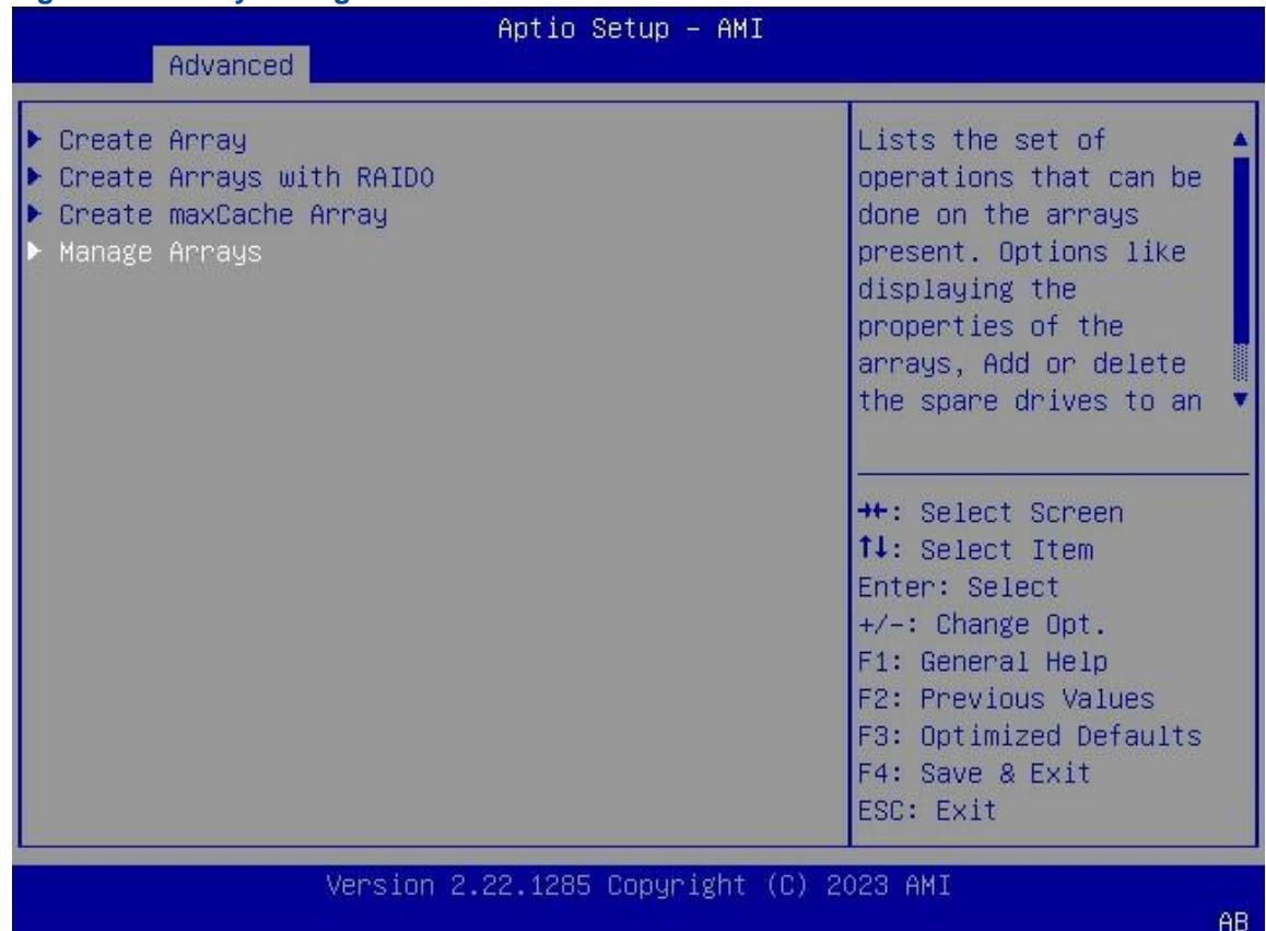
2. Use the arrow keys to select **Manage Arrays**, and then press **Enter**. The **Manage Arrays** screen is displayed, see [Figure 4-87](#).
