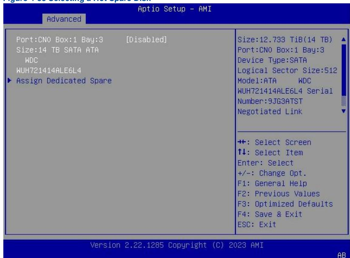
6. Use the arrow keys to select the disk to be set as a hot spare disk, press **Enter**, and then set the status of the disk to **Enabled**, see [Figure 4-84](#).
