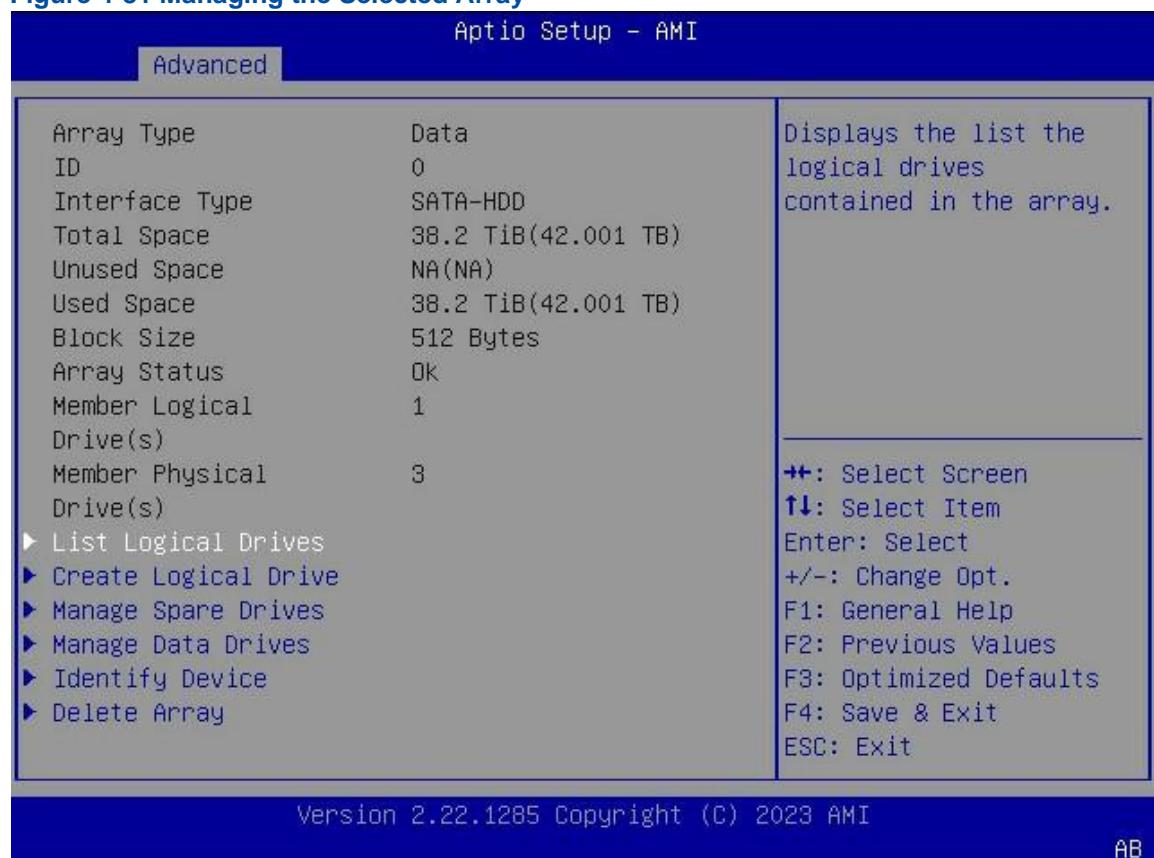
4. Use the arrow keys to select **Manage Spare Drives**, and then press **Enter**. The **Manage Spare Drives** screen is displayed, see [Figure 4-82](#).
