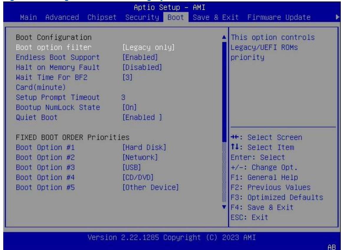
5. Press **F4** or use the arrow keys to select **Save & Exit > Save Changes and Exit**, and then press **Enter**. The **Save & Exit Setup** dialog box is displayed, see [Figure 5-6](#).
