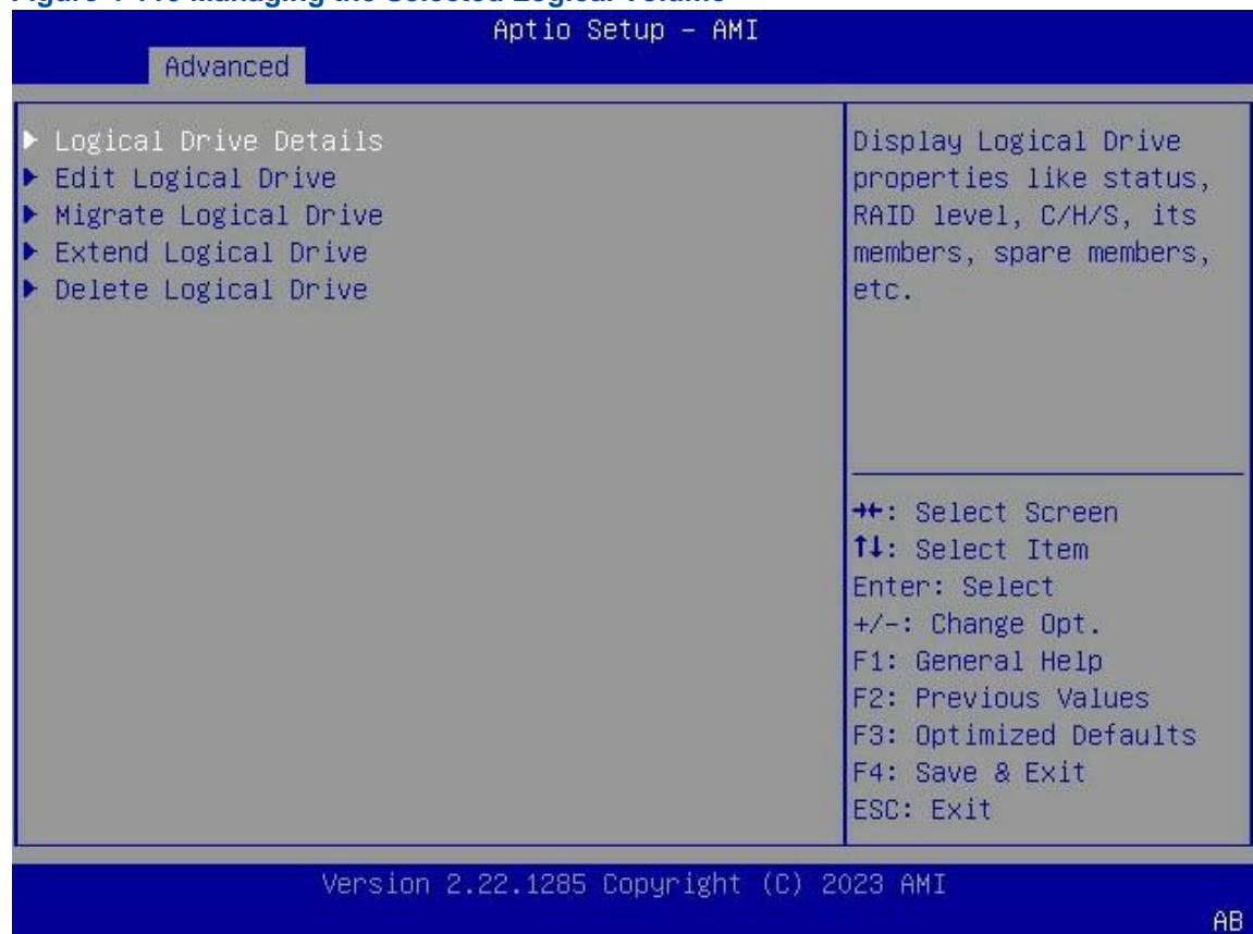
6. (Optional) To view the details of the logical volume, use the arrow keys to select **Logical Drive Details**, and then press **Enter**, see [Figure 4-111](#).
