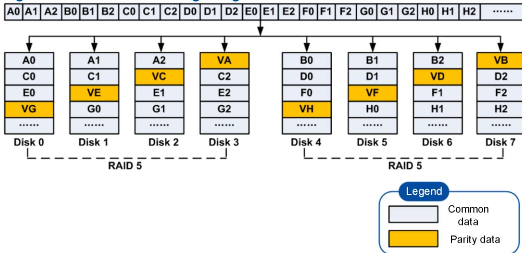
One RAID 50 array consists of multiple RAID 5 volumes. At least six hard disks are required for RAID 50. Data is distributed on each RAID 5 volume in RAID 0 mode.
