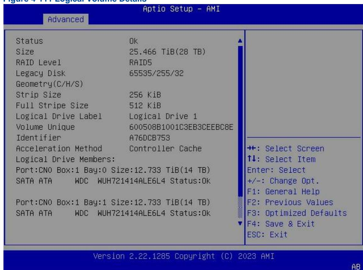
7. On the logical volume management screen, use the arrow keys to select **Delete Logical Drive**, and then press **Enter**. The confirmation screen for RAID volume deletion is displayed, see [Figure 4-112](#).
