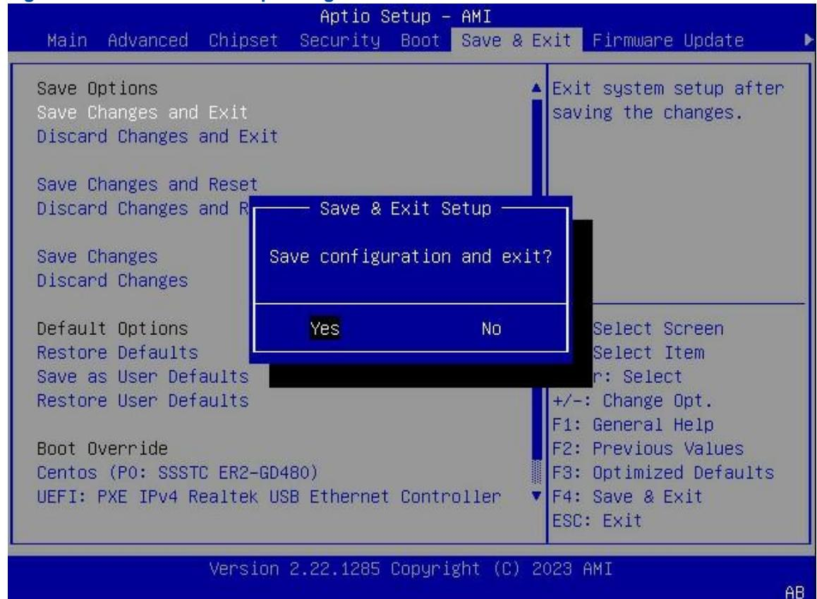
6. Use the arrow keys to select **Yes**, and press **Enter**. The boot mode is set to **UEFI**, and the server is restarted automatically.
