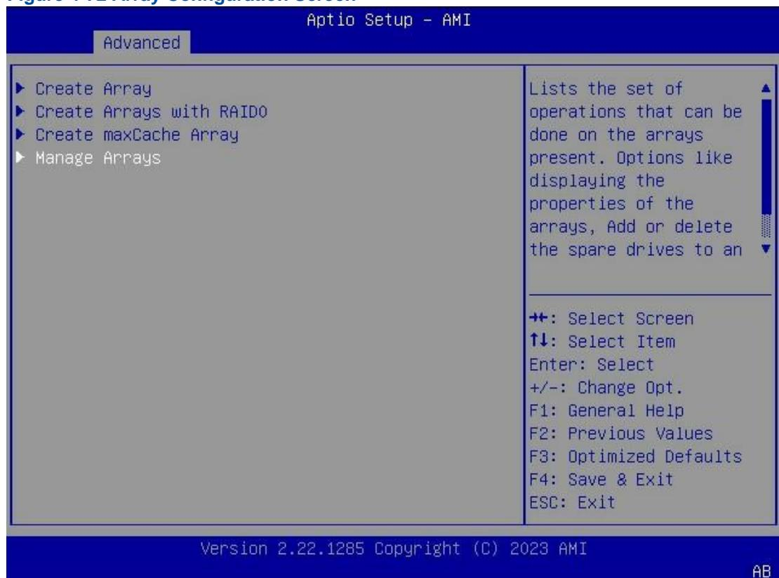
2. Use the arrow keys to select **Manage Arrays**, and then press **Enter**. The **Manage Arrays** screen is displayed, see [Figure 4-73](#).
