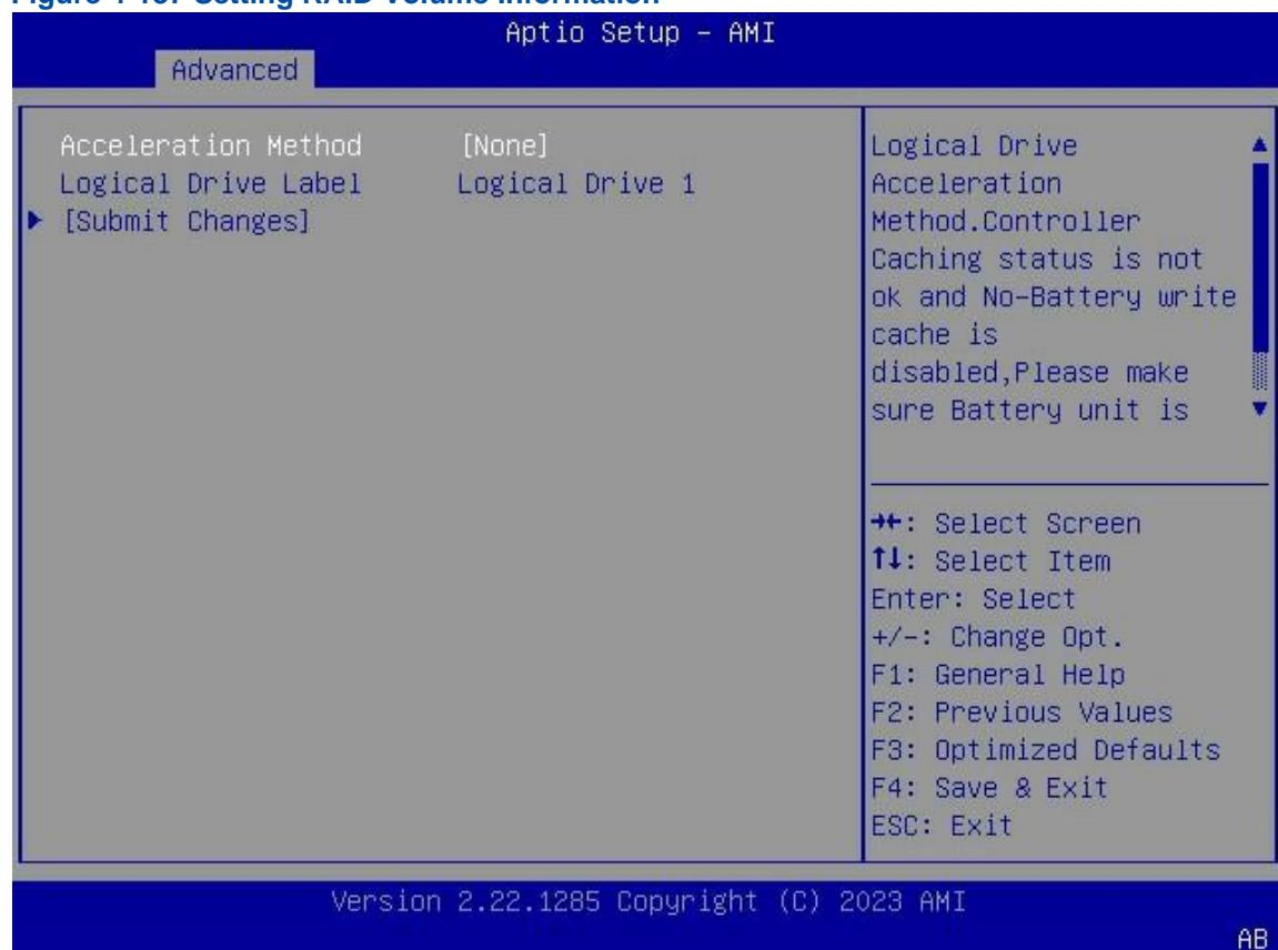
8. Use the arrow keys to select **Acceleration Method**, and then press **Enter**. The **Acceleration Method** dialog box is displayed, see [Figure 4-138](#).
