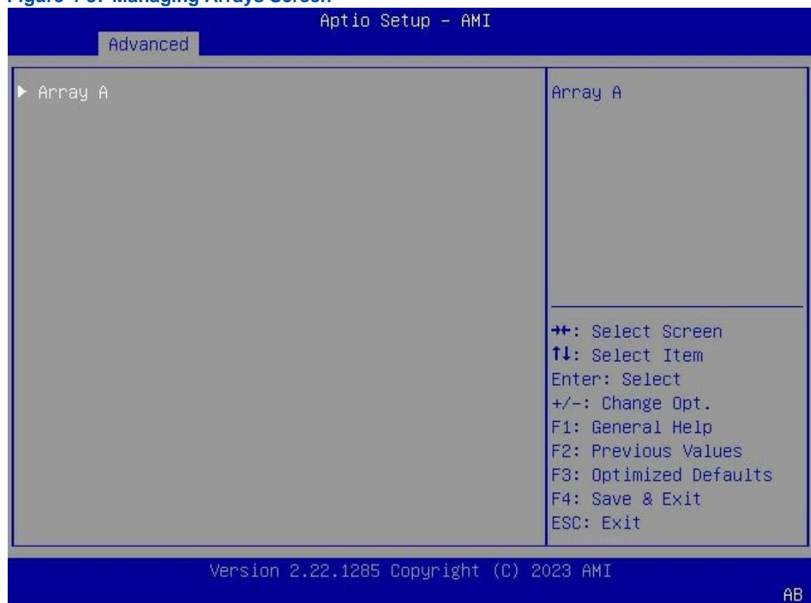
3. Use the arrow keys to select the array for which you need to modify the hot spare disk, and then press **Enter**. The screen for managing the selected array is displayed, see [Figure 4-88](#).
