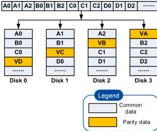
RAID 5 uses the [CRC](#) mode to distribute sequential data (A0–A2, B0–B2, C0–C2, D0–D2, ...) and the corresponding parity data (VA, VD, ...) to different member disks respectively.
