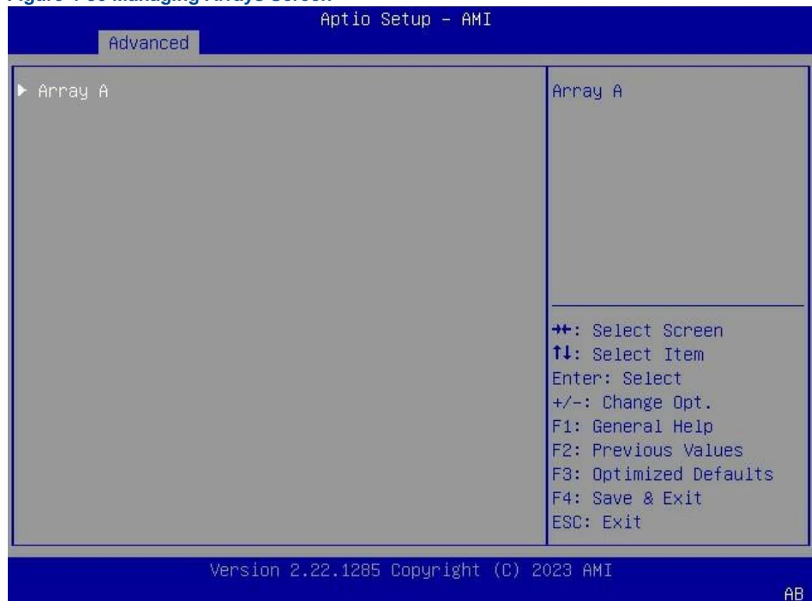
3. Use the arrow keys to select the array for which you need to create the hot spare disk, and then press **Enter**. The screen for managing the selected array is displayed, see [Figure 4-81](#).
