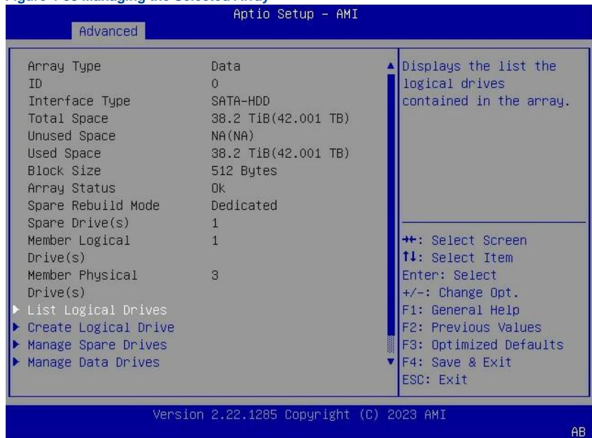
4. Use the arrow keys to select **Manage Spare Drives**, and then press **Enter**. The **Manage Spare Drives** screen is displayed, see [Figure 4-89](#).
