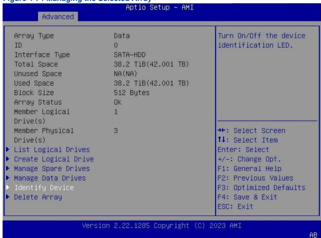
4. Use the arrow keys to select **Identify Device**, and then press **Enter**. The **Identify Device** screen is displayed, see [Figure 4-75](#).
