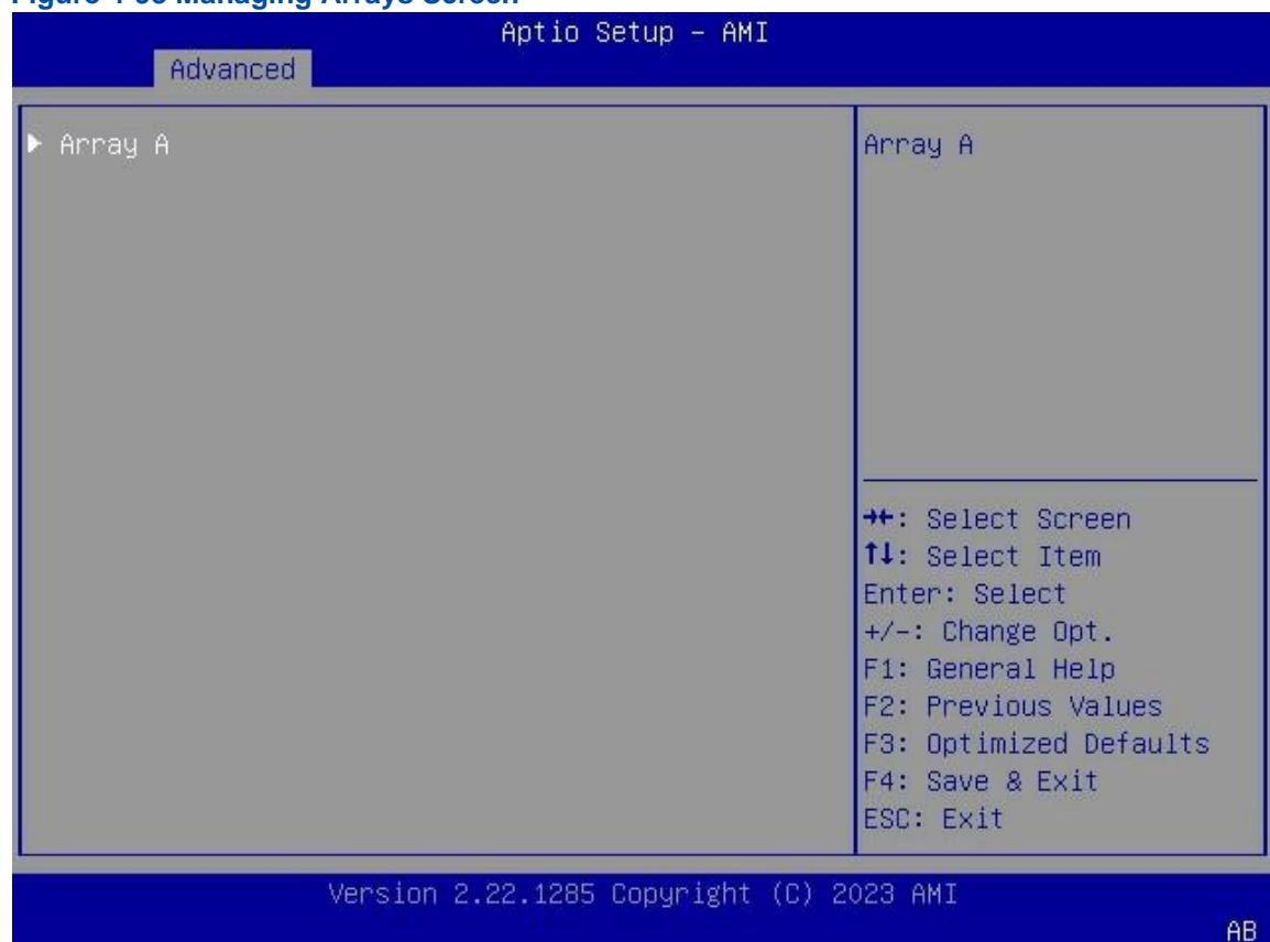
3. Use the arrow keys to select the array for which you need to delete the hot spare disk, and then press **Enter**. The screen for managing the selected array is displayed, see [Figure 4-94](#).
