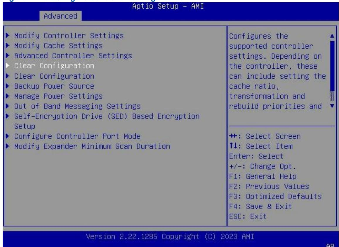
2. Use the arrow keys to select **Clear Configuration**, and then press **Enter**. The screen for clearing the configurations is displayed, see [Figure 4-120](#).
