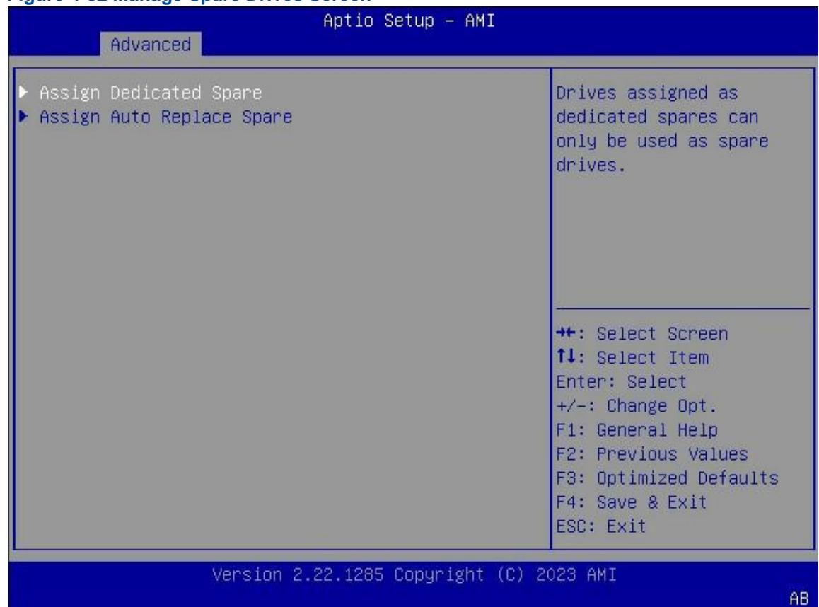
5. In accordance with your actual conditions, use the arrow keys to select the type of the hot spare disk to be created, and then press **Enter**. The screen for selecting a hot spare disk is displayed, see [Figure 4-83](#).
