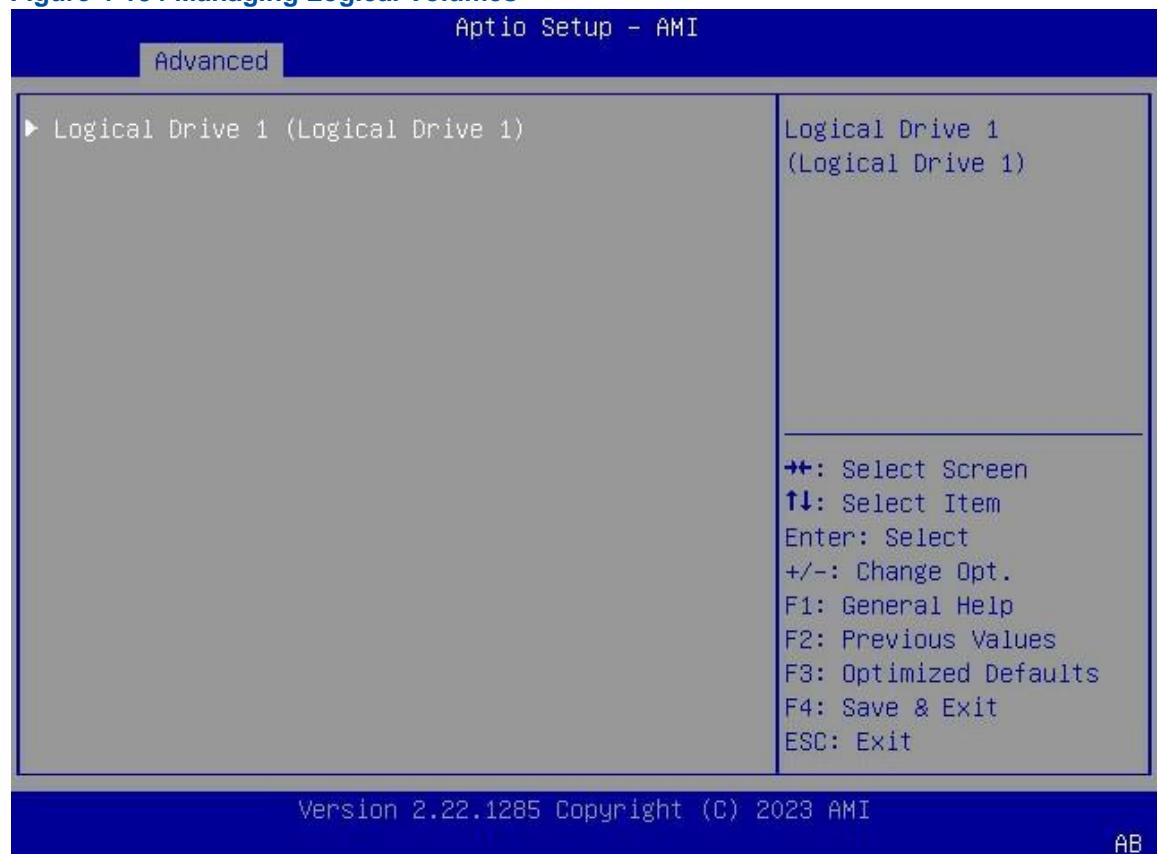
5. Use the arrow keys to select the RAID logical volume for which the caching function needs to be enabled, and then press **Enter**. The screen for managing the selected RAID logical volume is displayed, see [Figure 4-135](#).
