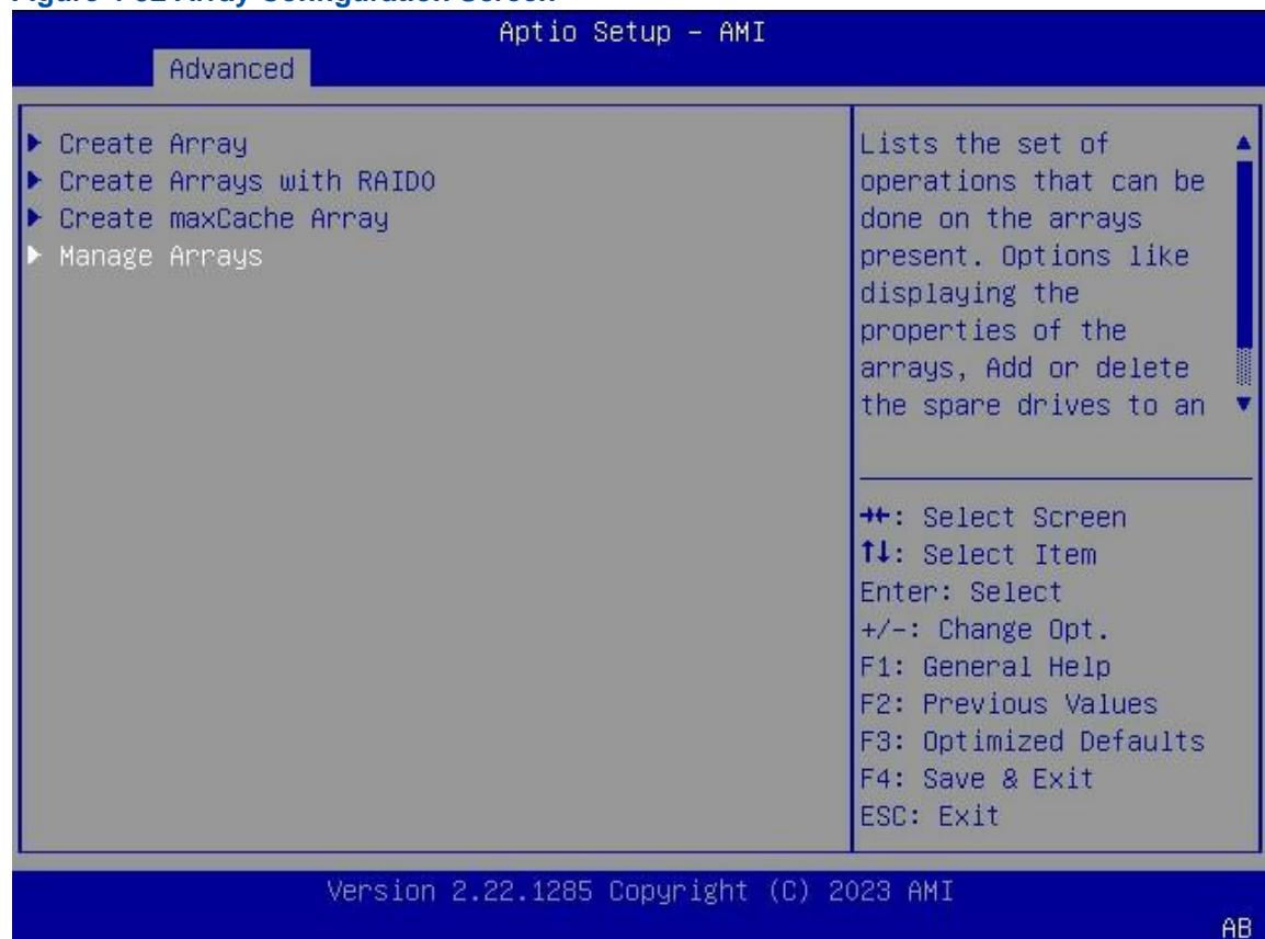
2. Use the arrow keys to select **Manage Arrays**, and then press **Enter**. The **Manage Arrays** screen is displayed, see [Figure 4-93](#).
