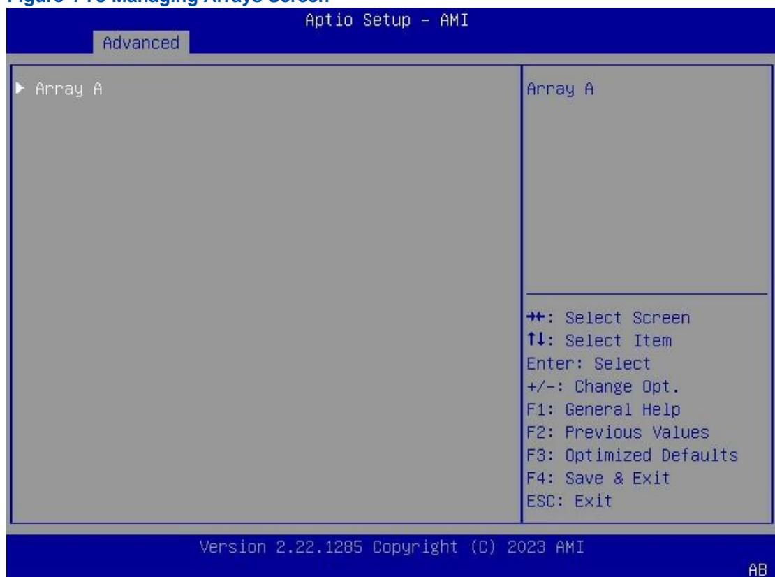
3. Use the arrow keys to select the array in which the disk to be located is placed, and then press **Enter**. The screen for managing the selected array is displayed, see [Figure 4-74](#).
