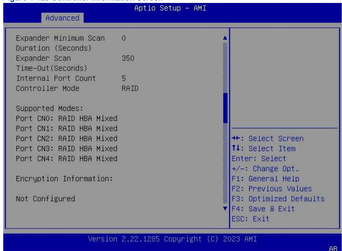
2. Press **Esc** to return to the controller management screen. Use the arrow keys to select **Configure Controller Settings**, and then press **Enter**. The **Configure Controller Settings** screen is displayed, see [Figure 4-124](#).
