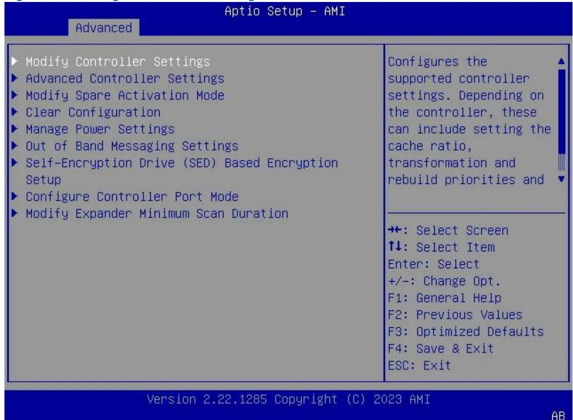
2. Use the arrow keys to select **Manage Power Settings**, and then press **Enter**. The **Manage Power Settings** screen is displayed, see [Figure 4-100](#).
