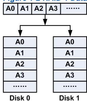
Each working disk of the RAID 1 array has a corresponding mirrored disk, and a piece of sequential data (A0, A1, A2, ...) needs to be written into the working disk and the mirrored disk respectively, which is equivalent to automatic backup.
