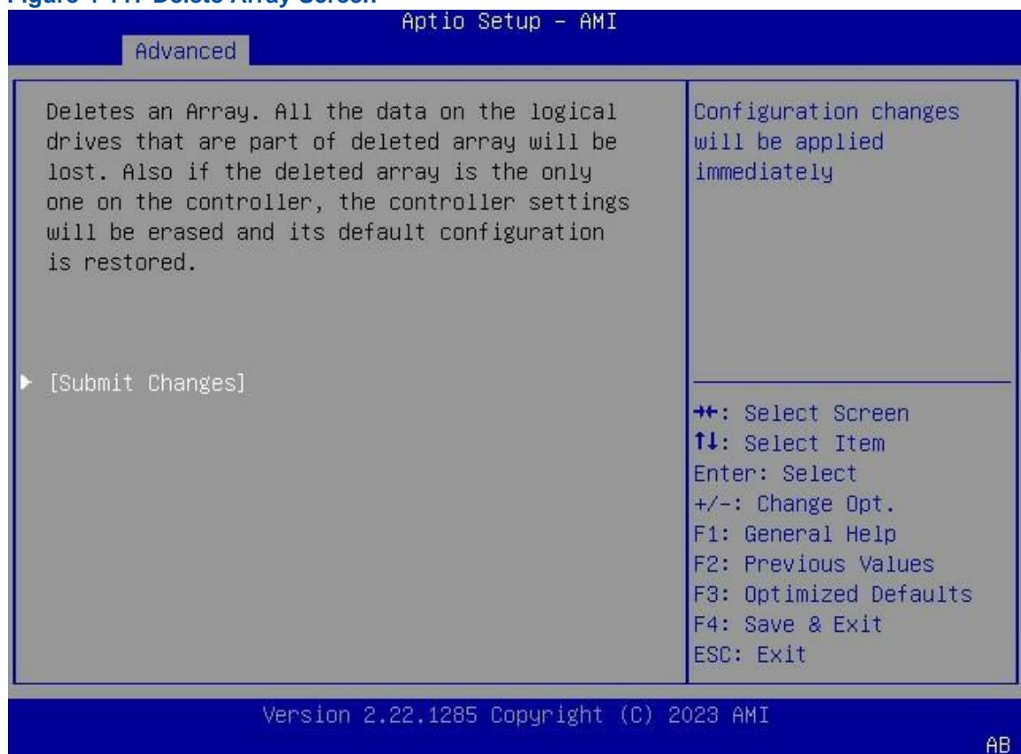
5. Use the arrow keys to select **Submit Changes**, and press **Enter**. The array is deleted successfully, see [Figure 4-118](#).
