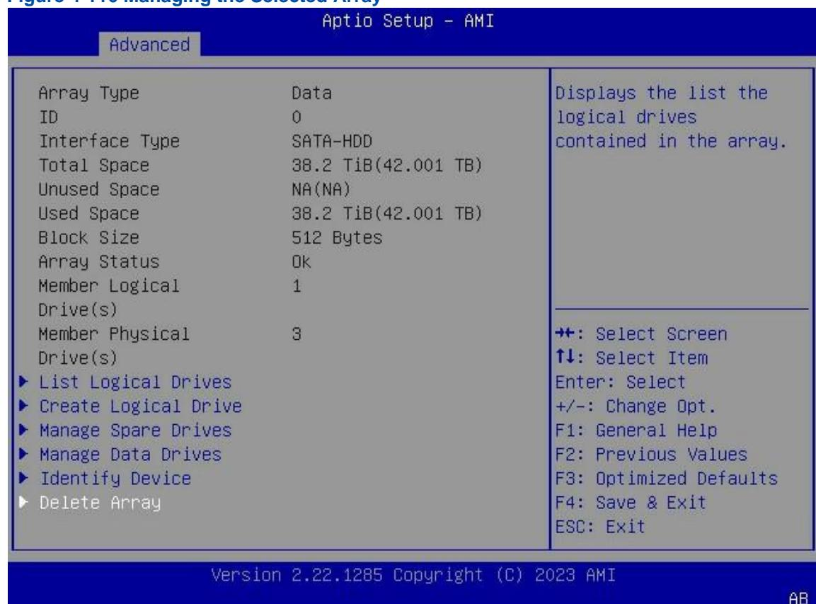
4. Use the arrow keys to select **Delete Array**, and then press **Enter**. The **Delete Array** screen is displayed, see [Figure 4-117](#).
