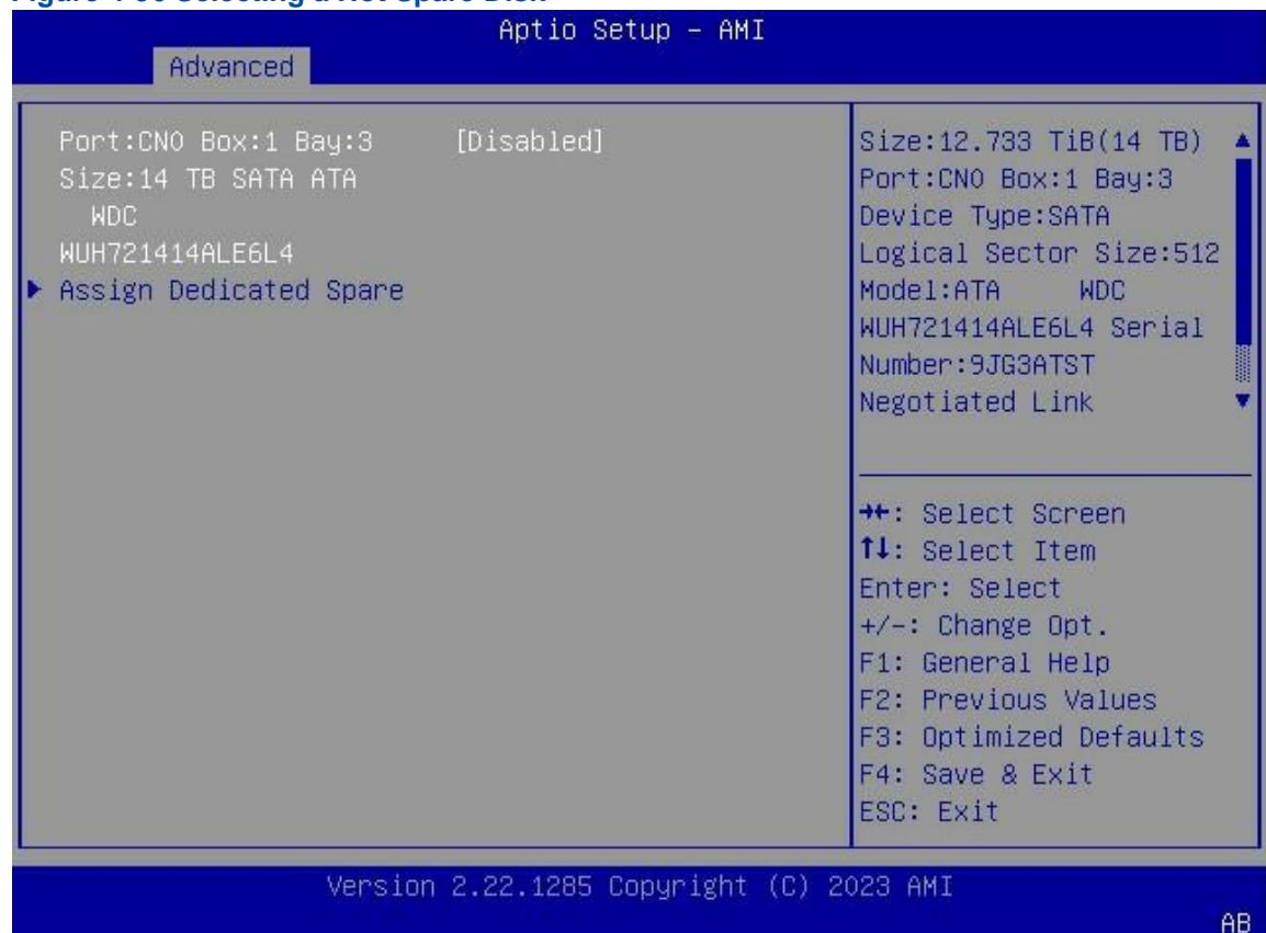
6. Use the arrow keys to select the hot spare disk to be deleted, press **Enter**, and then set the status of the disk to **Enabled**, see [Figure 4-97](#).
