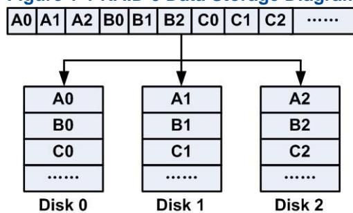
The storage principle of RAID 0 is to distribute sequential data (A0–A2, B0–B2, C0–C2, ...) to several member disks.
