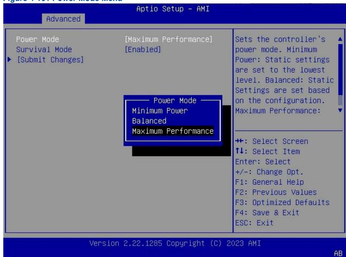
4. In accordance with your actual conditions, use the arrow keys to select the power mode to be applied, and then press **Enter** for confirmation, see [Figure 4-102](#).
