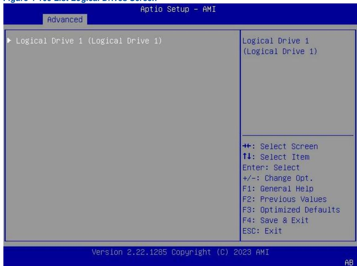
5. Use the arrow keys to select the logical volume to be deleted, and then press **Enter**. The screen for managing the selected logical volume is displayed, see [Figure 4-110](#).
