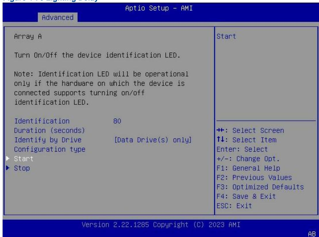
6. Use the arrow keys to select **Start**, and then press **Enter**. The status indicators of the member disks of the array are lit up solid blue (as shown in [Figure 4-77](#)).
