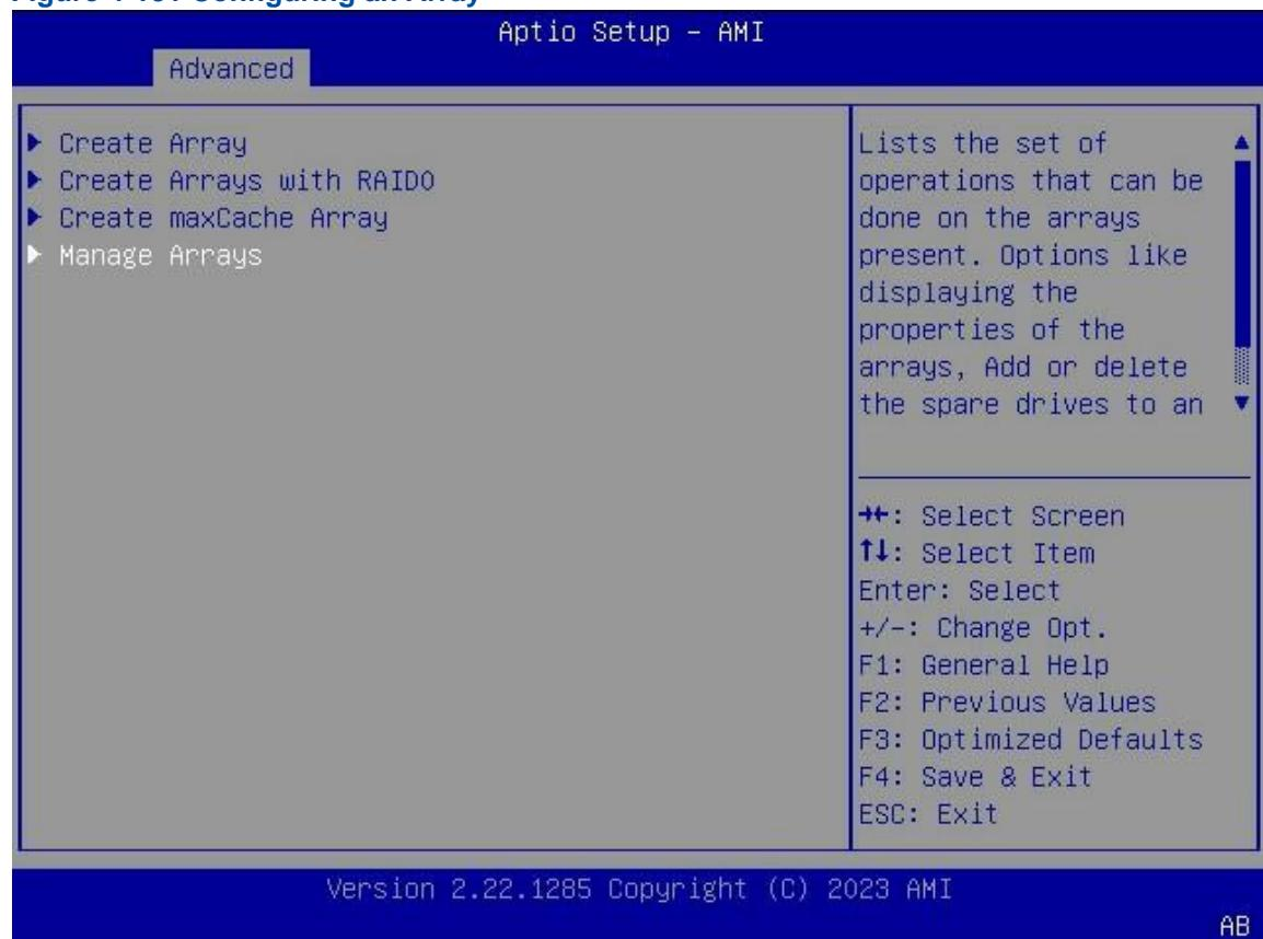
2. Use the arrow keys to select **Manage Arrays**, and then press **Enter**. The screen for managing arrays is displayed, see [Figure 4-132](#).
