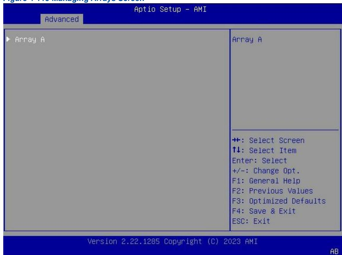
3. Use the arrow keys to select the array to be deleted, and then press **Enter**. The screen for managing the selected array is displayed, see [Figure 4-116](#).
