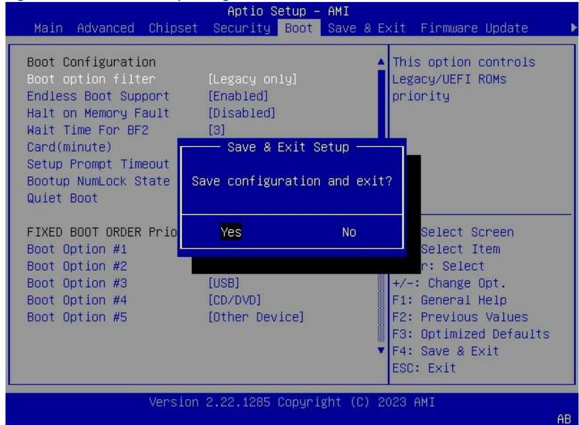
6. Use the arrow keys to select **Yes**, and press **Enter**. The boot mode is set to **Legacy**, and the server is restarted automatically.
