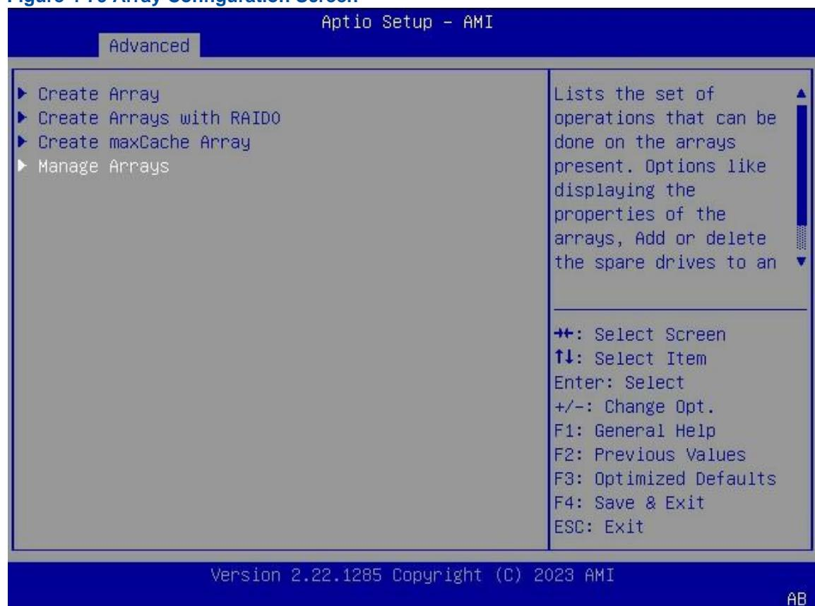
2. Use the arrow keys to select **Manage Arrays**, and then press **Enter**. The **Manage Arrays** screen is displayed, see [Figure 4-80](#).
