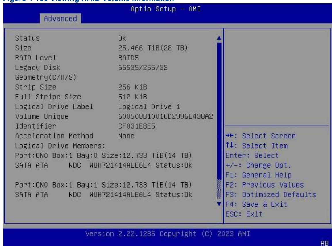
7. Press **Esc** to return to the RAID volume management screen. Use the arrow keys to select **Edit Logical Drive** and press **Enter**. The screen for setting RAID volume information is displayed, see [Figure 4-137](#).
