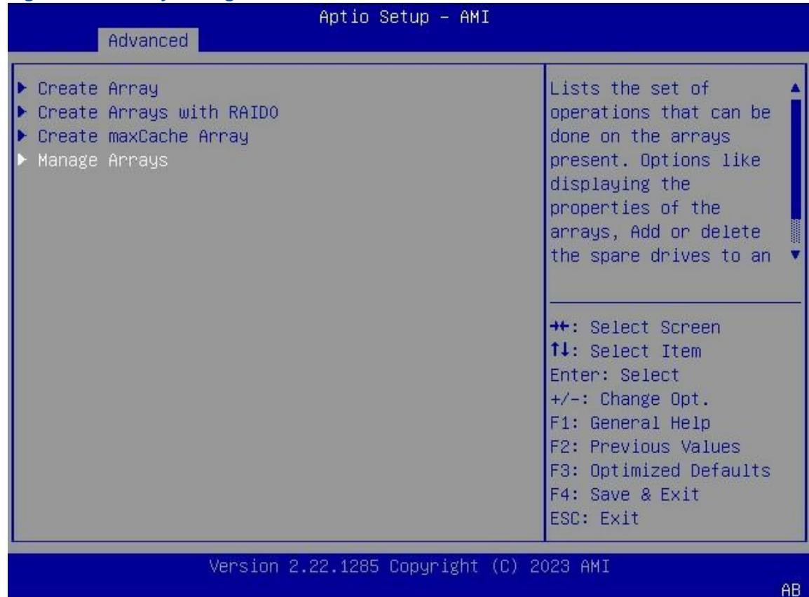
2. Use the arrow keys to select **Manage Arrays**, and then press **Enter**. The **Manage Arrays** screen is displayed, see [Figure 4-115](#).
