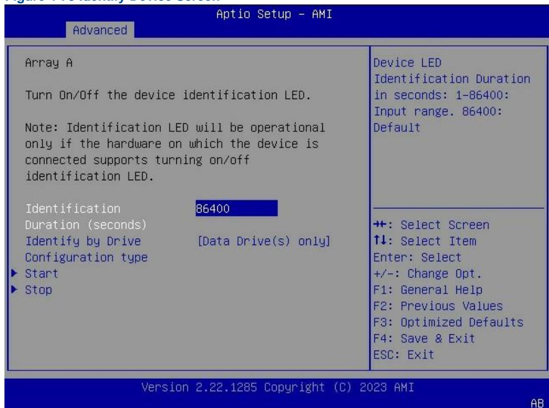
5. Next to **Identification Duration (seconds)**, enter the time of the lighting delay (unit: seconds), and then press **Enter** for confirmation, see [Figure 4-76](#).
