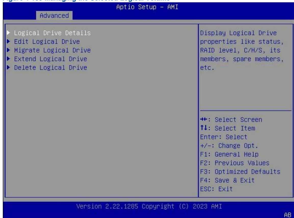
6. Use the arrow keys to select **Logical Drive Details**, and press **Enter**. The RAID volume information is displayed, see [Figure 4-136](#). The value of **Acceleration Method** is **None**, indicating that the caching function is disabled.
