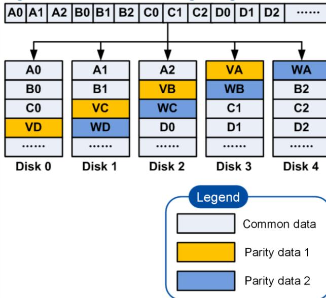
Like RAID 5, RAID 6 distributes sequential data (A0–A2, B0–B2, C0–C2, D0–D2, ...) and the corresponding parity data (VA, VD, ...) to different member disks respectively.
