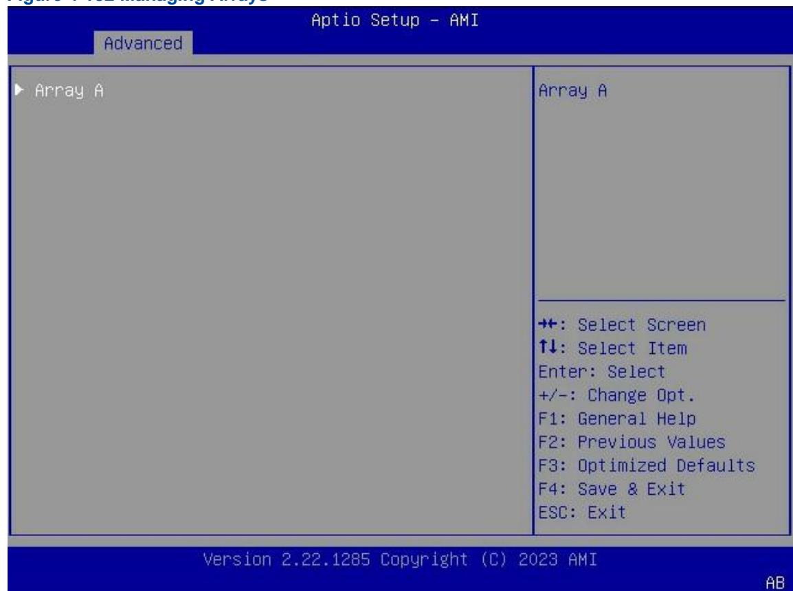
3. Use the arrow keys to select the array for which the caching function needs to be enabled, and then press **Enter**. The screen for managing the selected array is displayed, see [Figure 4-133](#).
