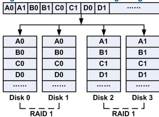
RAID 10 can be regarded as: Two member disks in a pair (Disk 0 and Disk 1, Disk 2 and Disk 3, ...) form a multiple RAID 1 volume. Multiple RAID 1 volumes form a RAID 0 array, and data is distributed on each RAID 1 volume in the form of RAID 0.
