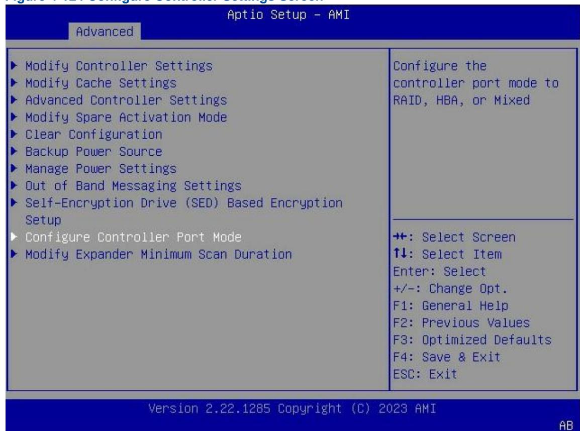
3. Use the arrow keys to select **Configure Controller Port Mode**, and then press **Enter**. The screen for setting the port mode is displayed, see [Figure 4-125](#).
