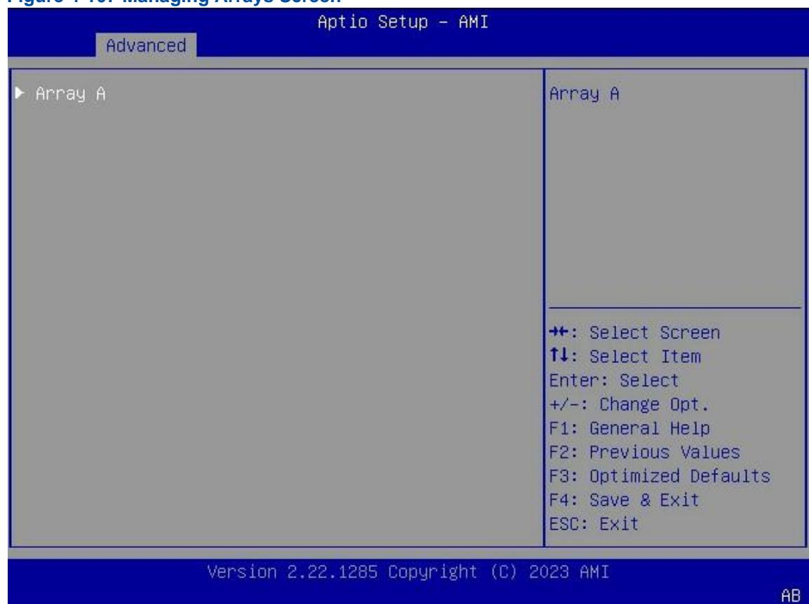
3. Use the arrow keys to select the array for which you need to delete a logical volume, and then press **Enter**. The screen for managing the selected array is displayed, see [Figure 4-108](#).
